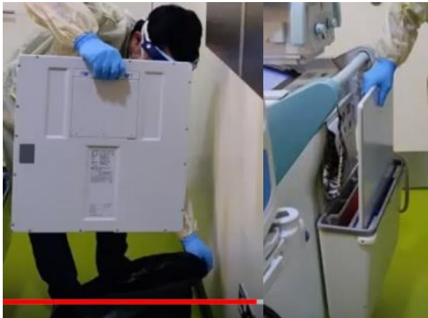
9. Remove detector from sleeve, place in machine's detector stand, discard the sleeve and sanitise the gloved hand
