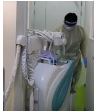
10. Move machine into anteroom, sanitise gloved hands Clean and disinfect the machine and detector At last remove PPE as per institute guidelines
